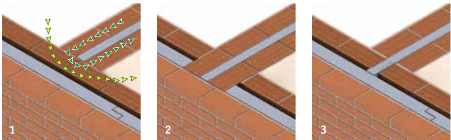
(E) – Some configurations of the connection between the internal dividing wall and the front double-layered wall made of clay elements.
