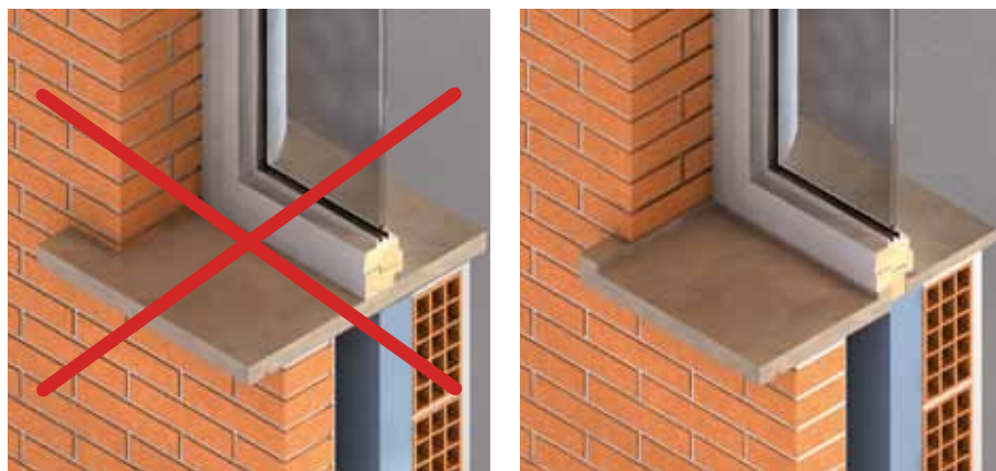
(C) – Solving of a thermal bridge in the connection point between the window frame – sill – opaque closure by detachment from the external sill in coincidence with the insulating layer.
